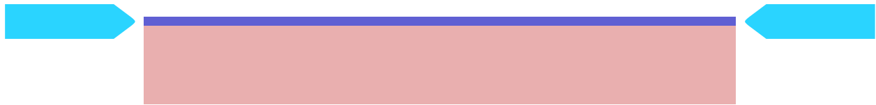
(a) LW device coupling scheme : the waveguide (dark blue) is as long as the sample
