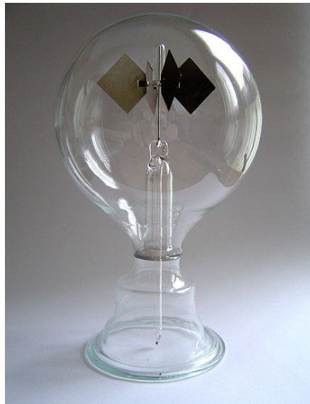
Figure 1 – Crooke's light mill. The vanes rotate on a low friction spindle and vacuum is made in the glass bulb. The vanes are black on one side, and mirror coated on the other. If light is shone on the apparatus from one direction, photons impinging on the black side of a vane will be absorbed, resulting on a momentum transfer of \hbar k per photon ( k is the wavenumber of the photon), while those impinging on a mirror coated side will be reflected, resulting in a momentum transfer 2\hbar k . This net difference is in theory accountable for the rotation of the vanes. In first experiments though, the vanes were rotating in the wrong direction, because of thermal effects. Crookes invented this radiometer in 1873 but one had to wait 1901 to see an experimental demonstration of radiation pressure with such a device.
