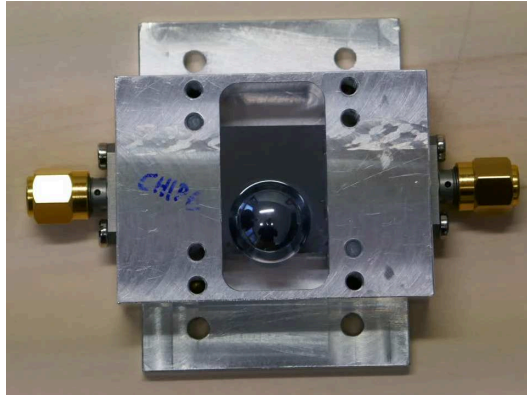
Figure 7.4.1: Chip_6 illuminated side with the lens mounted. Because of its size, it has been necessary to enlarge the chip holder window.
