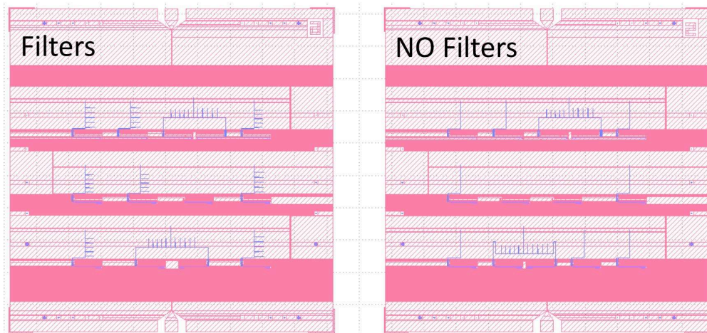
Figure 6.4.3: Two versions of the same LEKID geometry, one with filters and the other with the antenna directly coupled to the LEKID. The two dual color pixels have filters in any case due to the nature of the diplexer.
